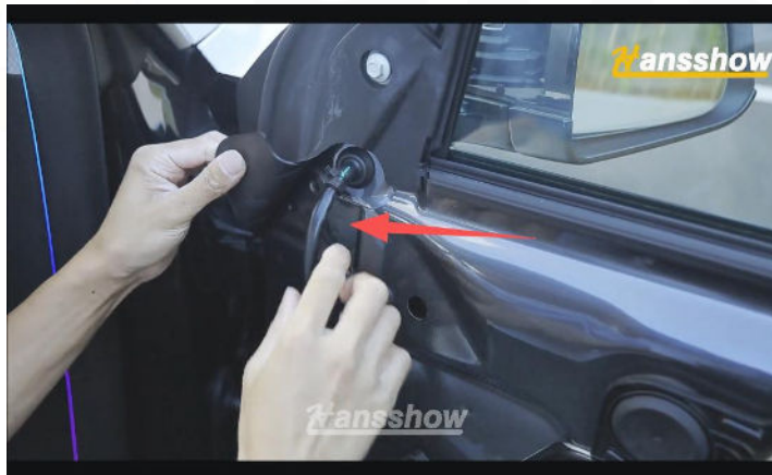
11. Remove the rubber plug covering the side mirror mounting screws (same for both sides).
