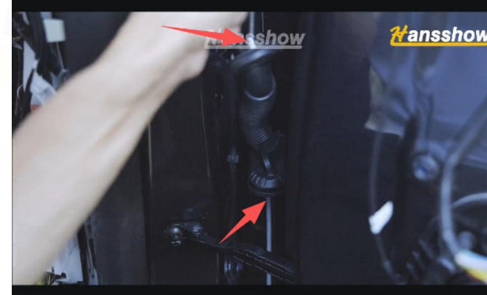
32.Pass the wire guide through the rubber waterproof tube.
