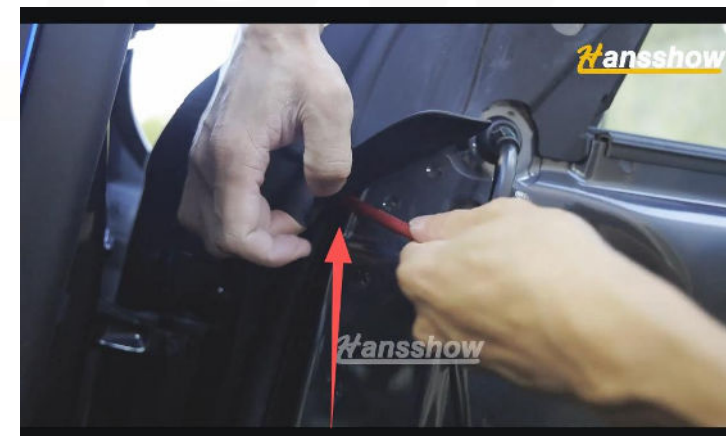
12. Unclip the side mirror rubber trim (same for both sides).
