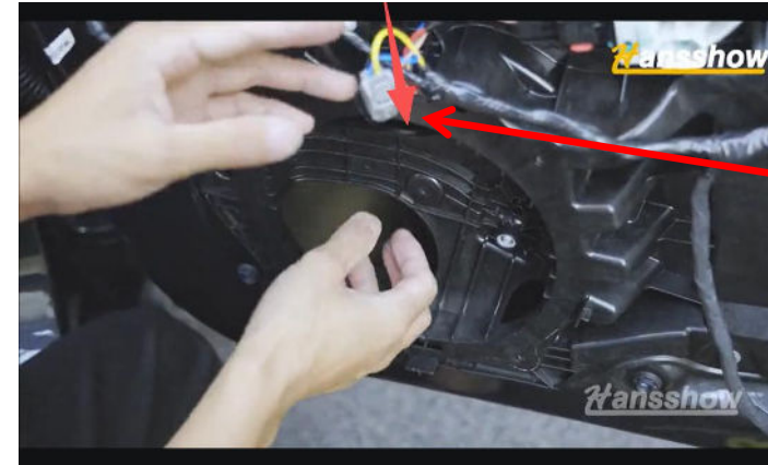
30.Route one end of the right-side power cable to the rubber waterproof tube.
