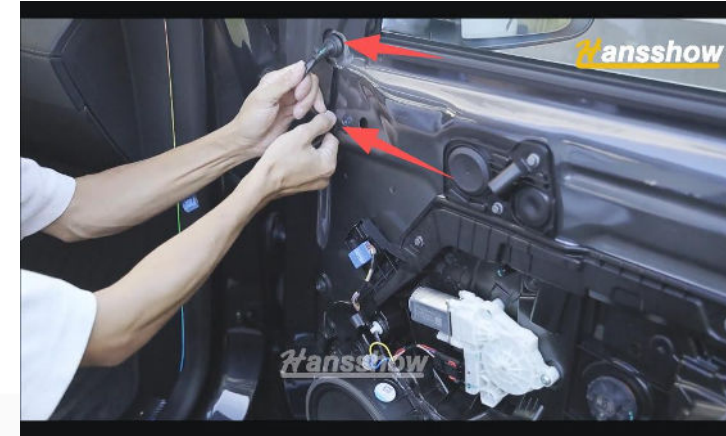
10. Remove the side mirror wiring harness clip (same for both sides).
