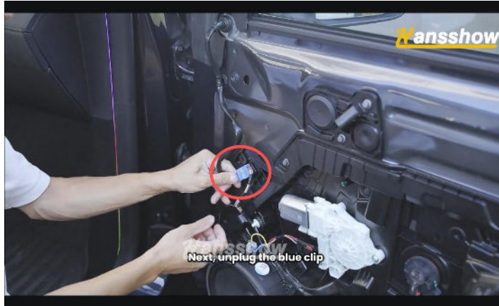
9. Unplug the side mirror connector (same for both sides).
