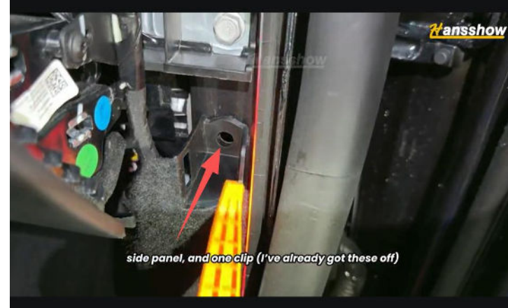
5. Remove the door sill trim clips.
