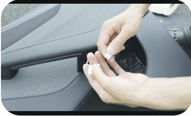
10. Connect the armrest light to the power cable.
