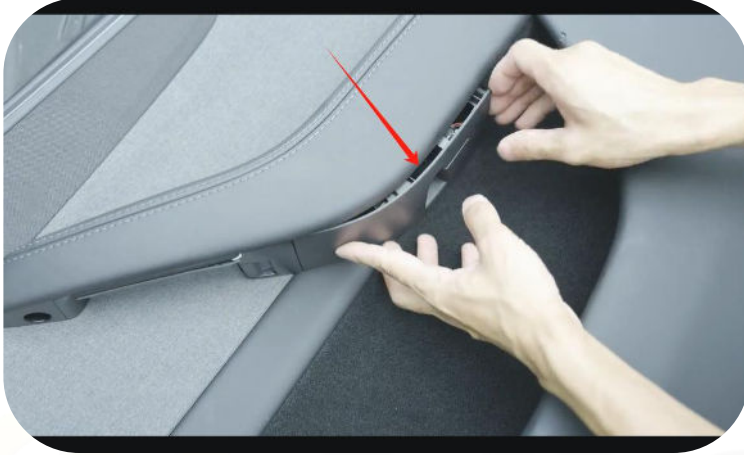
15. Reinstall the trim under the handle.
