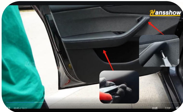
3. Unscrew front-facing door panel screws.
