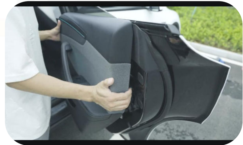
13. Reinstall the door panel and screw it back.
