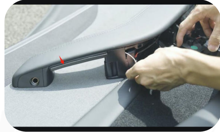
12. Stick the lower part of the light onto the handle.
