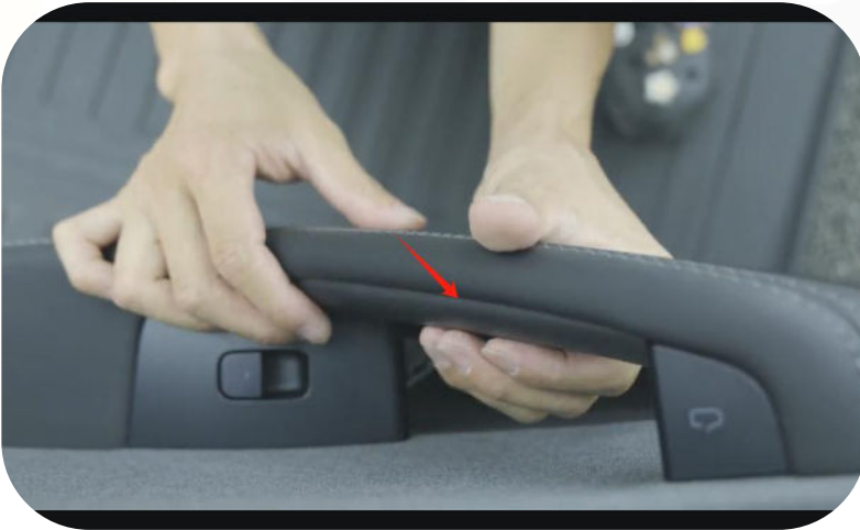
8. Insert the top side of the light into the gap, and stick the bottom side to the handle.
