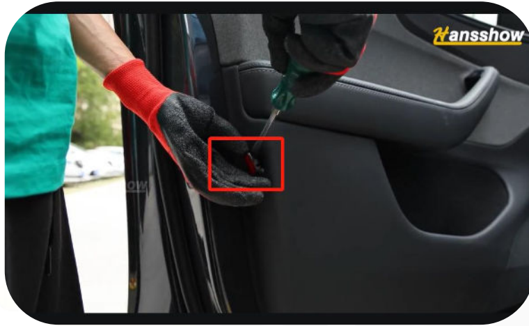
1. Remove red decorative cover on the side of the front door.
