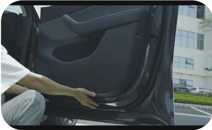
17. Reinstall and screw the door panel back in place.
