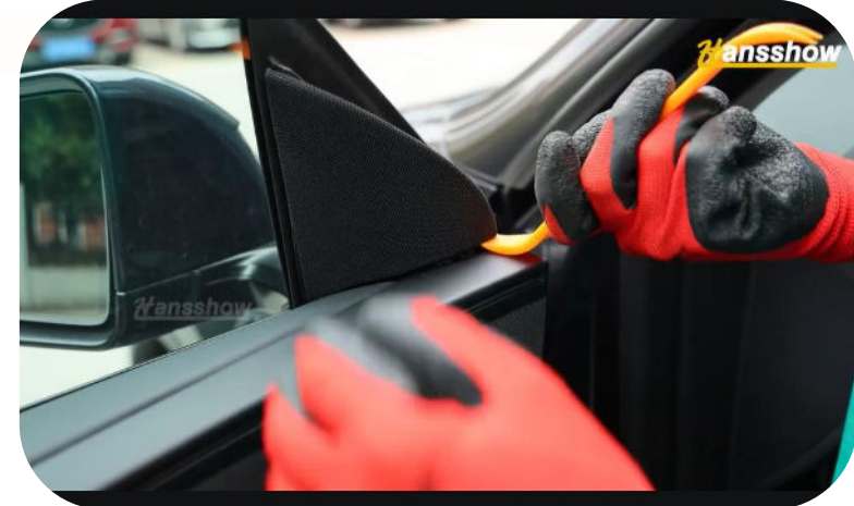
4. Remove the tweeter speaker.
