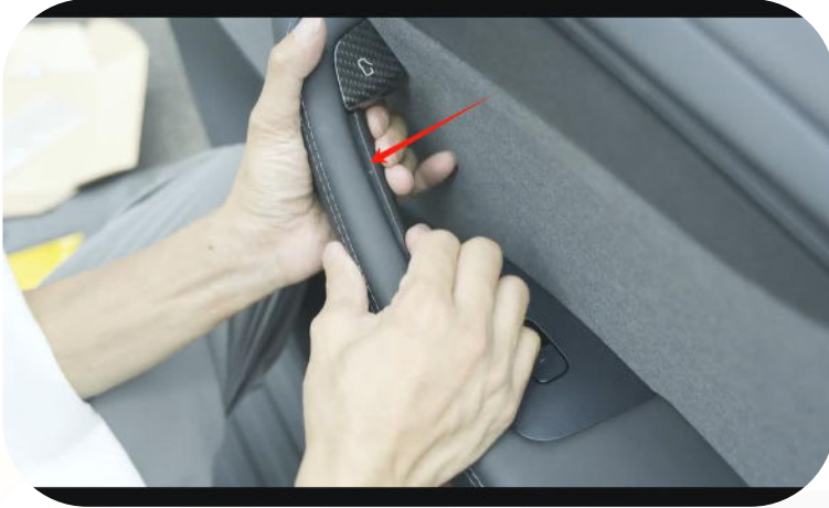
11. Clip the top part of the light into the door handle gap.
