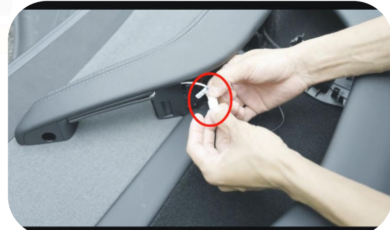
14. Connect the armrest light to the power cable.
